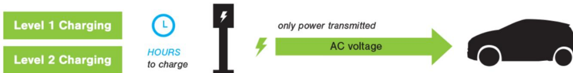
FIGURE 4—LEVELS 1 AND 2 SLOW CHARGING AC
