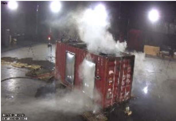
TR propagation after water flow off [TR + 01:13:05]
