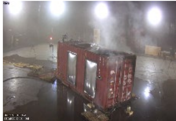
TR propagation continues after water flow restart [TR + 01:49:54]
