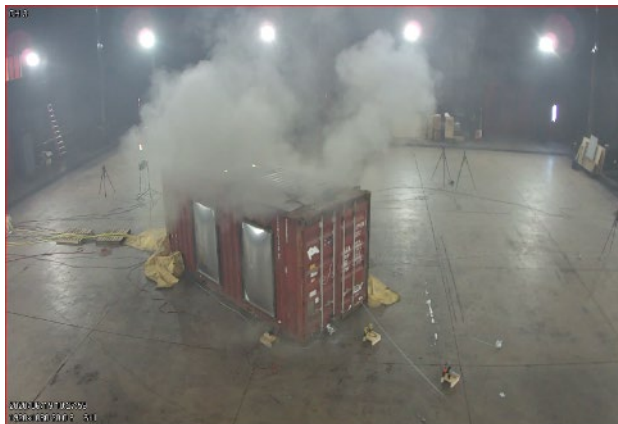
TR propagation for 3 hours [TR + 00:11:54]
