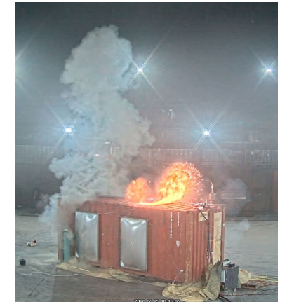
UL 9540A installation test
