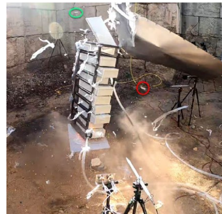
UL 9540A unit test
