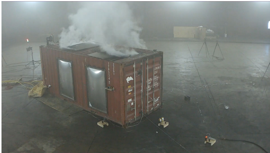
UL's tests — flashover
