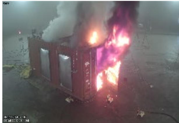
Flashover conditions and flaming from open door [TR + 02:09:48]
