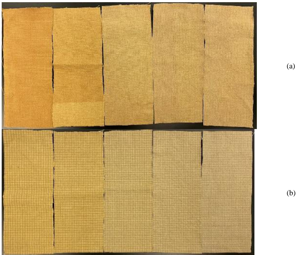
Figure 6.9: Visual change of fabric from 0 wash (far left) to 100 washes (far right) for the (a) 2003 and (b) 2017 turnout materials. From left to right in each picture the specimens are 0, 1, 25, 50, 100 wash cycles.
